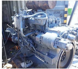
Panashe and Mhaka overhauled the Bulldozer engine and gave it a respray when they were done
